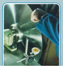
The final sharpening angle is ground onto the blade and before they are packed into wooden cases they are finally tested for axial run-out as shown.
