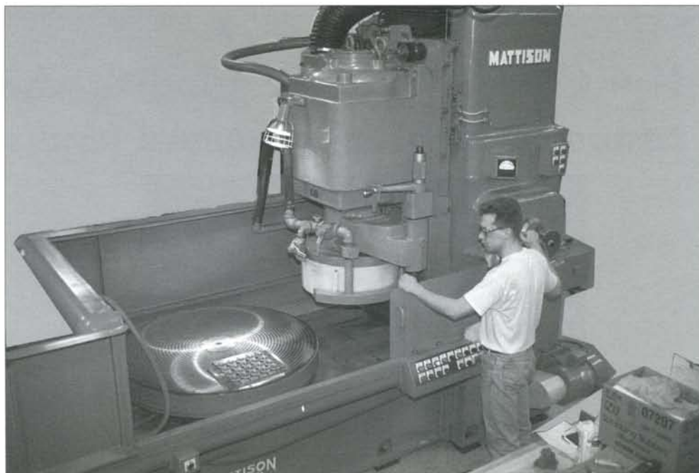
Cash Masters works with our new Mattison rotary grinder. It has a larger table and more spindle horsepower than our older Blanchard grinder. The machine is a real workhorse in removing heavy stock.
