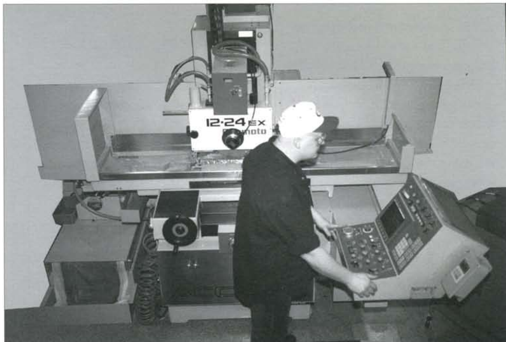
Dave Muschinski operates our new Okamoto surface grinder with all of the latest features: a 5-horsepower spindle with variable speeds up to 1800 RPM, a Fanuc 2-axis CNC control, a fully automatic diamond dresser with dress compensation, and automatic wheel balancing.
