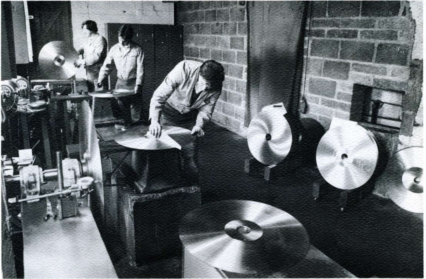
Microblade smithers applying their special Sheffield craft to the manufacture of log saw blades.
