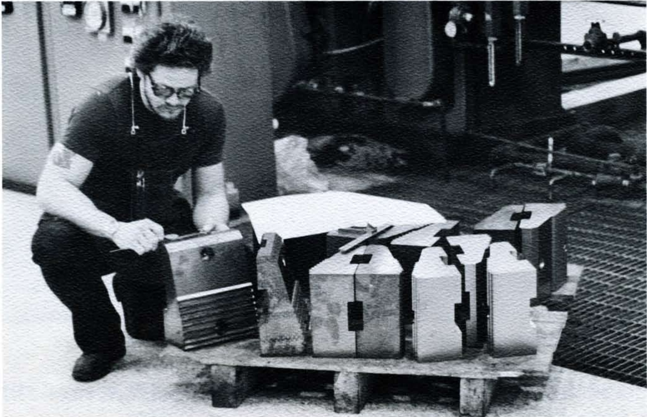
Ron Olson, Kinetic's milling department leadman, verifying lifter shoe hole location prior to heat treating.
