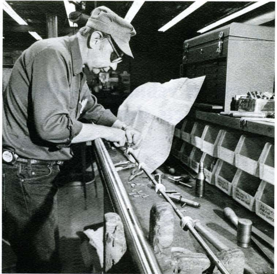
Ray Gwitt, known around Kinetic as "The Mandrel Doctor," replaces the worn fingers (dogs or pins) on a mandrel. Ray selects the right replacement parts by referring to the assembly drawing.
