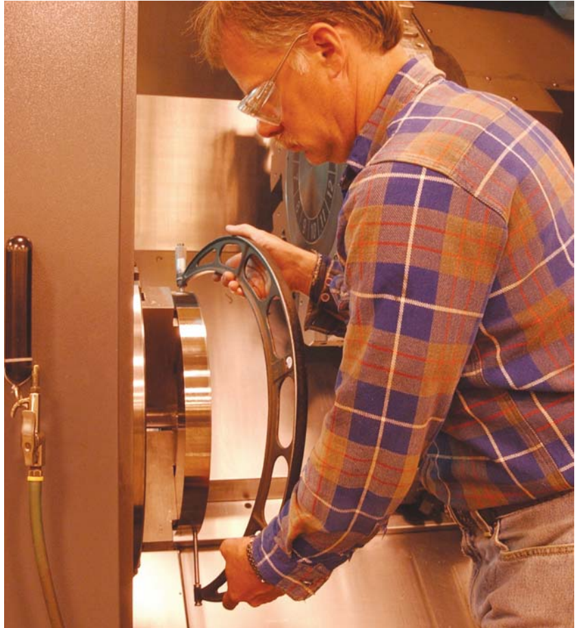
Jeff Kulinski loads a part into Kinetic's NL2000 turning center with subspindle and bar feeder.
